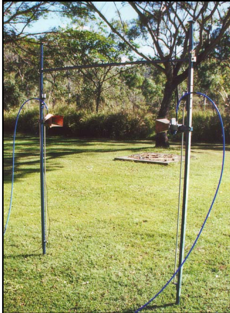
Figure 3.2: Portable testing unit showing the worm drive mounts used to vary the transmission height of the horn antennas.
