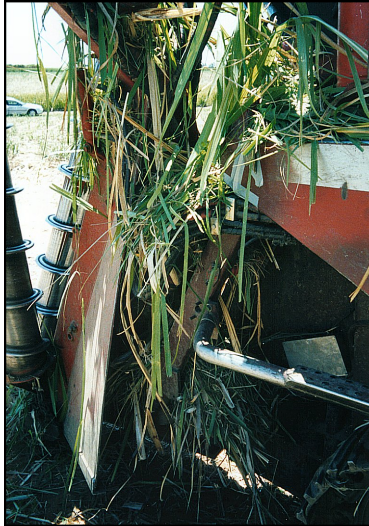
Figure 1.8: Photograph of trash caught behind the row divider of the Austoft R & D harvester after harvesting.
