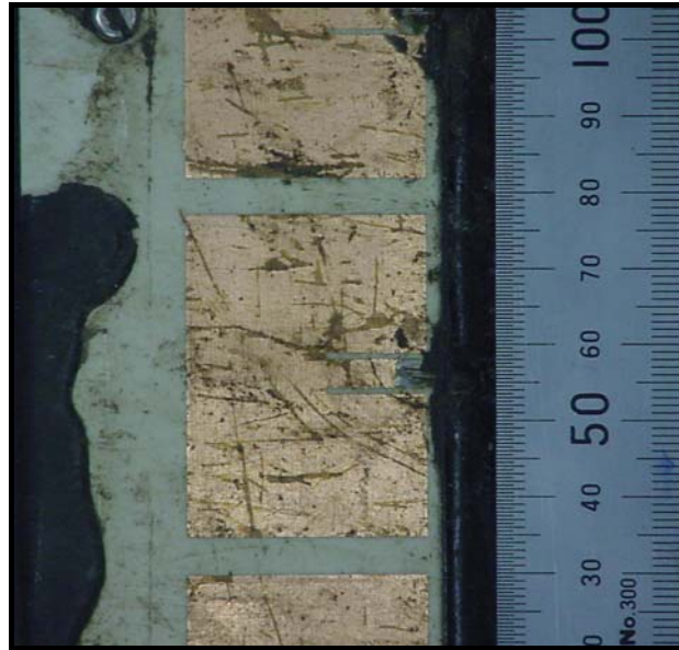
Figure 4.5: Photograph of the surface of the receiver antenna after one week of operation on a sugar cane harvester
