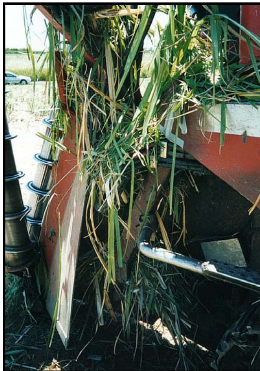
Figure 4.7: A photograph of the trash caught behind the row divider cavity after 15 minutes of operation
