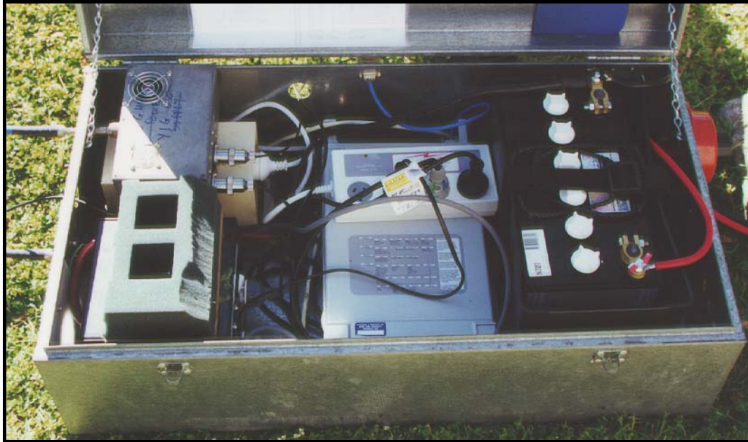
Figure 3.3: Photograph of the control box showing the YIG microwave source, Anritsu power meter, power inverter and 12 volt battery
