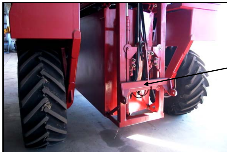
Figure 3.24: Photograph of the back of a high clearance tractor showing the height adjustable mount
