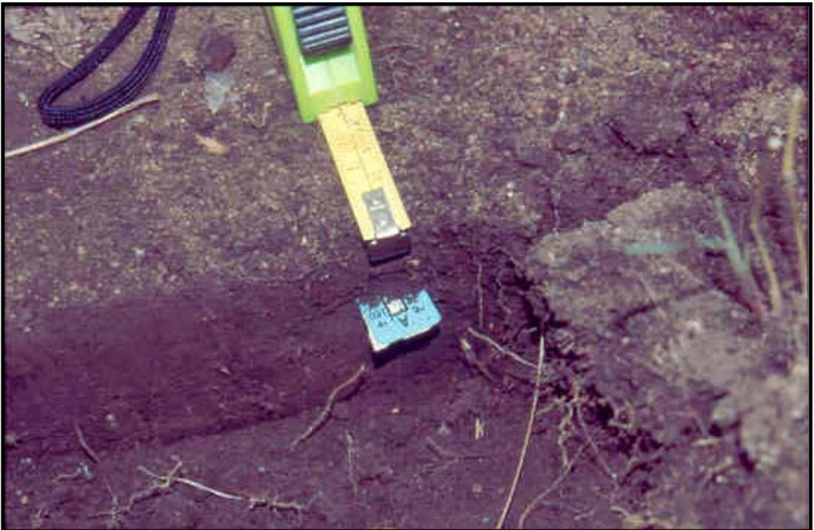
**Figure 4.4.** Placement of a temperature measurement strip at the 30 mm depth.
