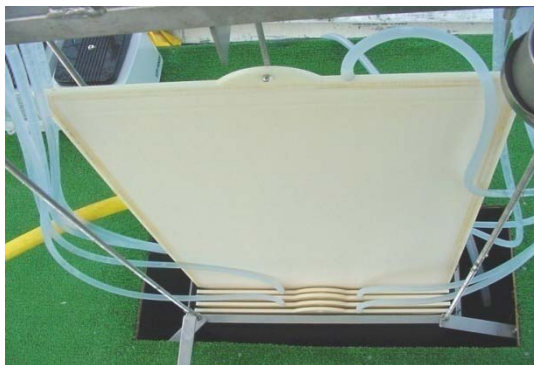
Fig. 3.11 New membrane sheet
